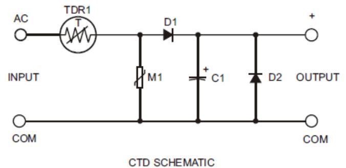
These devices are protected against inadvertent short circuits, input from line surges and inductive kickback from trip coils.
